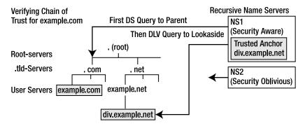
Figure 11-7. DLV verification procedure
